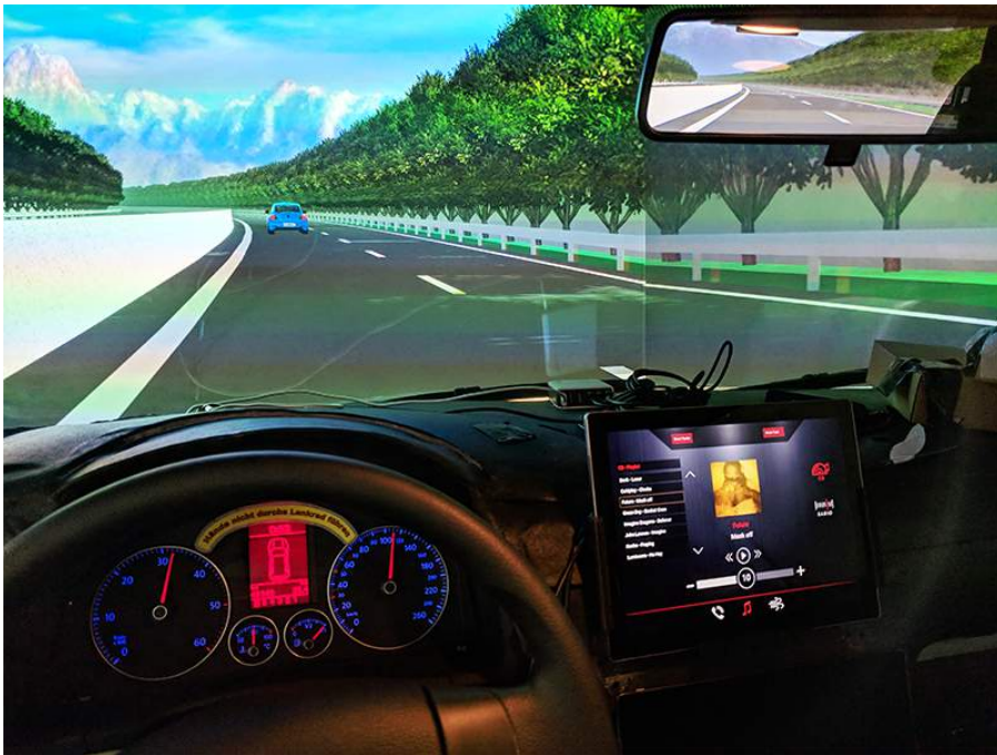
Figure 5.3: Study setup showing the driving scenario and an example of the IVIS used to investigate the interaction between UX and trust.
